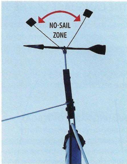
The masthead fly shows the direction of the apparent wind.
